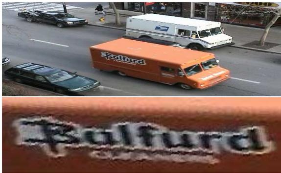
**Figure 7.** Most text are parallel to the vehicle body. The moving vehicle is extracted from the scene and oriented horizontally before applying the text detection algorithm. The angle of rotation can be derived using the angle of the vehicle's parallel edges, the direction of travel, or prior knowledge of the scene. The "Balfurd" image shows what the text looks like after rotation.
