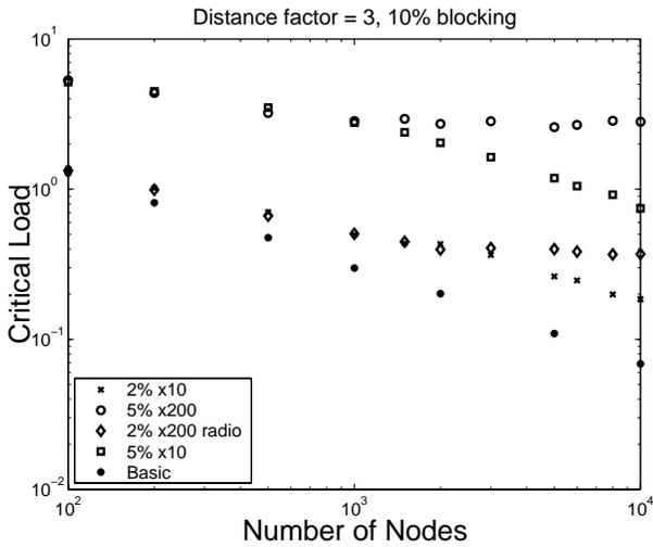
Figure 4: Comparison for different meganode parameter sets. Note, that function values for the  $x = 0.05$  case are multiplied by 3 for better visualization.
