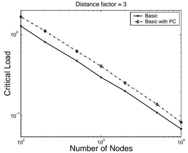
Figure 1: Comparison plot for 10% blocking. The increase with power control is about +35%.
