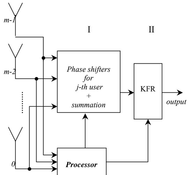
**Fig. 1** Functional scheme of the configuration with RAKE receivers
