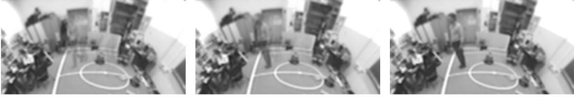
Figure 2: An example of the evolution of the dynamic background. From left to right a stationary person is gradually merged into the static background.
