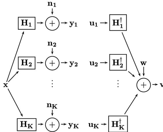
Fig. 2. System models of the MIMO BC(left) and the MIMO MAC (right) channels
