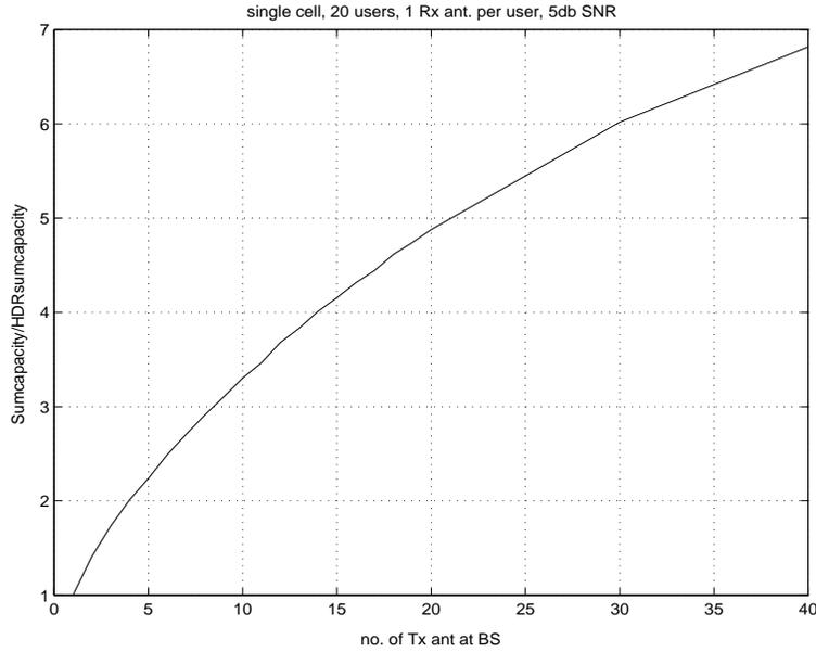
Fig. 6. Optimal Sum Rate relative to HDR
