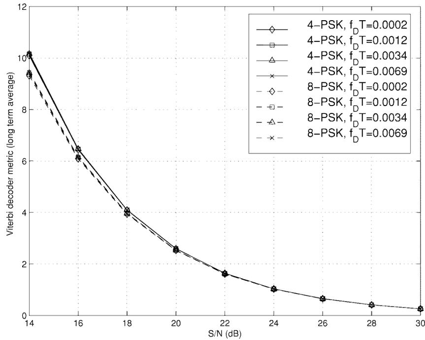
Fig. 4. Long-term average of Viterbi decoder metric versus  $S/N$  for rate 5/6 convolutionally coded coherent PSK (no interferers).
