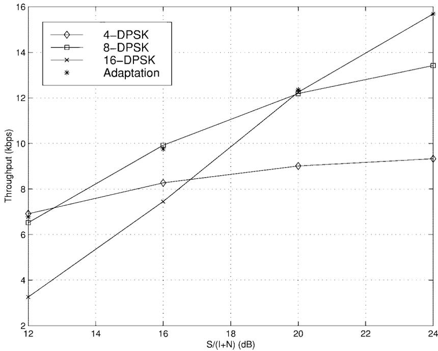
Fig. 11. Throughput for slow feedback-based rate adaptation in interference limited conditions;  $f_d T = 0.0002$ .
