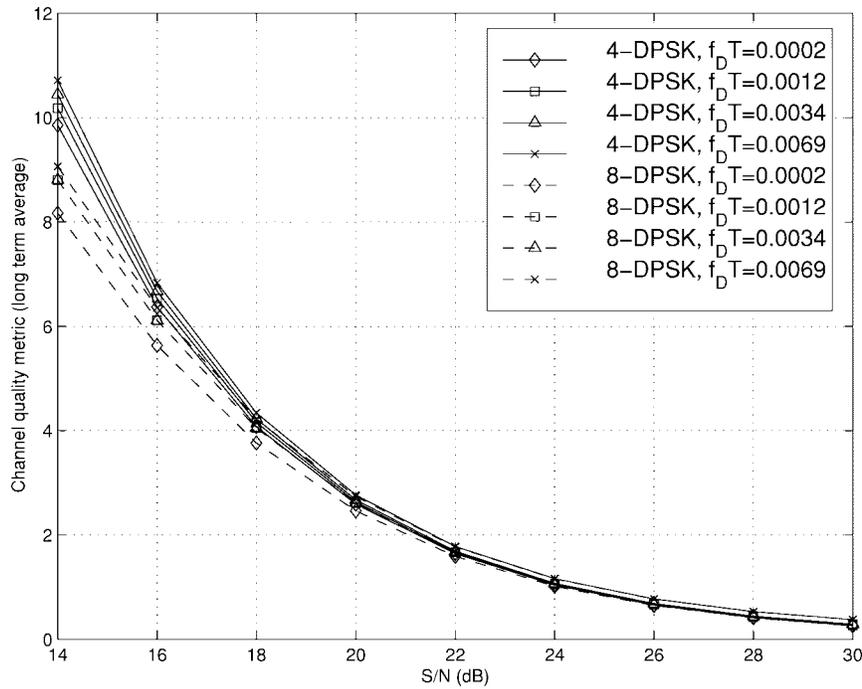
Fig. 5. Long-term average of scaled ED metric versus  $S/N$  for rate 5/6 convolutionally coded differential PSK (no interferers).
