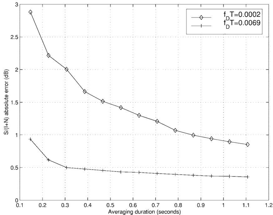
Fig. 8.  $S/(I+N)$  estimation error as a function of averaging duration for different Dopplers; rate 5/6 convolutionally coded 4-DPSK,  $S/(I+N) = 16$  dB,  $I/N = 10$  dB, differential detection, no CSI.
