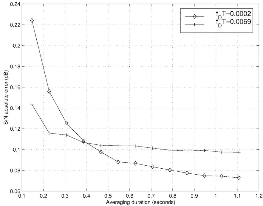
Fig. 7.  $S/N$  estimation error as a function of averaging duration for different Dopplers; rate 5/6 convolutionally coded 4-DPSK,  $S/N = 16$  dB, differential detection, no CSI.
