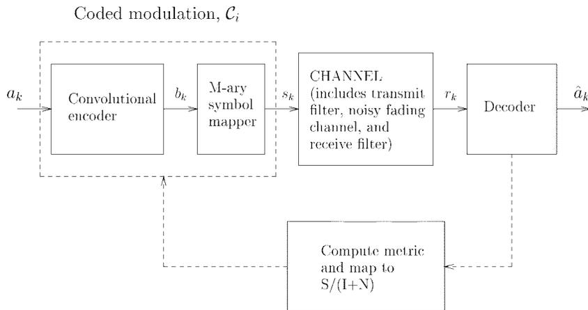
Fig. 1. Block diagram of system: equivalent baseband representation. Receiver provides channel quality feedback to the transmitter.  $a_k$ : information sequence;  $b_k$ : coded sequence;  $s_k$ : symbol sequence;  $r_k$ : received sequence;  $\hat{a}_k$ : decoded sequence.
