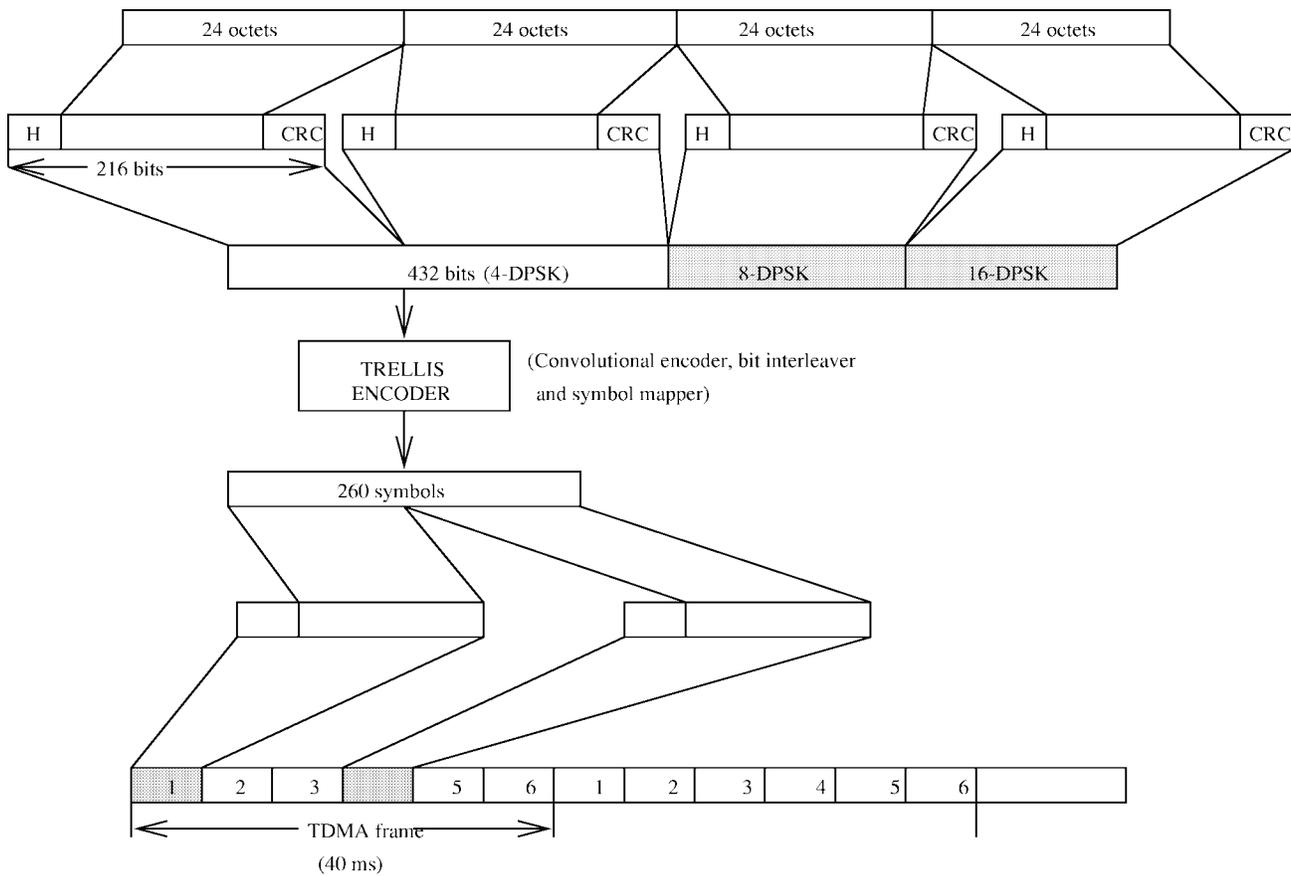
Fig. 2. Packing of multiple data frames into a time-slot pair.
