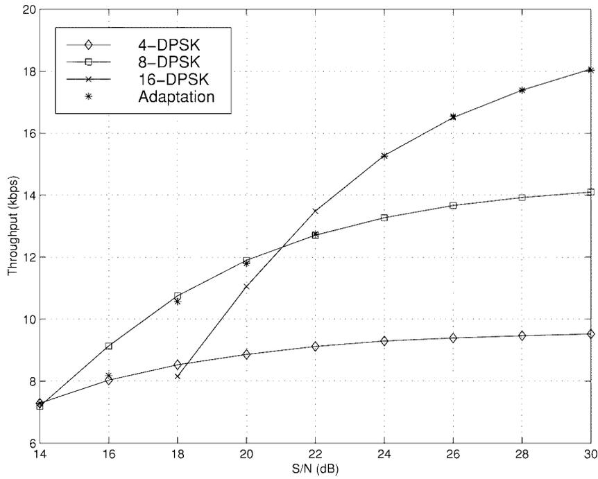
Fig. 9. Throughput for slow feedback-based rate adaptation in noise limited conditions;  $f_D T = 0.0002$ .
