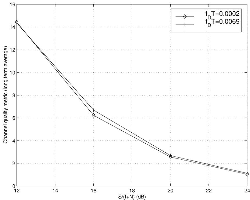
Fig. 6. Long-term average of scaled ED metric versus  $S/(I+N)$  for rate 5/6 convolutionally coded 4-DPSK (differential detection, no CSI,  $I/N = 20$  dB); the metric is consistent across Dopplers even with fading interferers.
