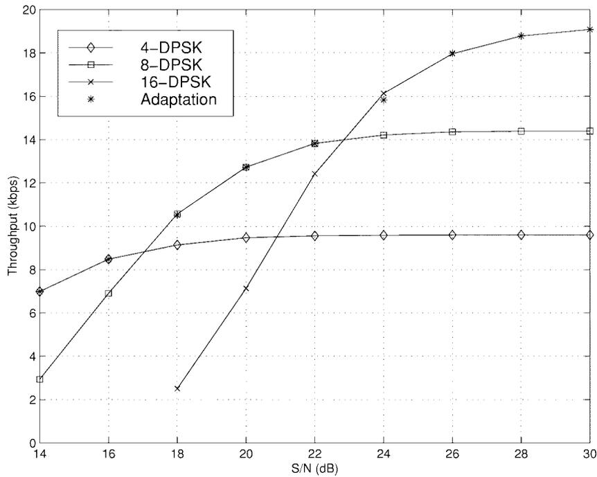
Fig. 10. Throughput for slow feedback-based rate adaptation in noise limited conditions;  $f_D T = 0.0069$ .
