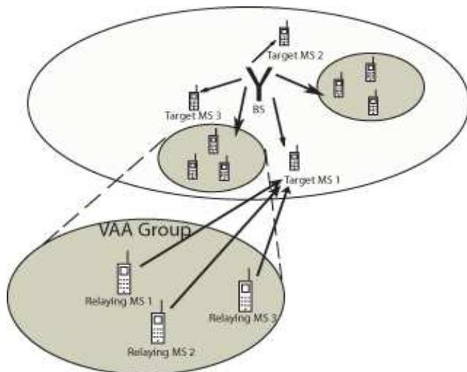
Fig. 1. Virtual Antenna Array System
