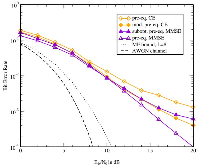
Fig. 3. Performance of CE, mod-CE, MMSE and suboptimal MMSE pre-equalization techniques, spreading length  $L=8$ .
