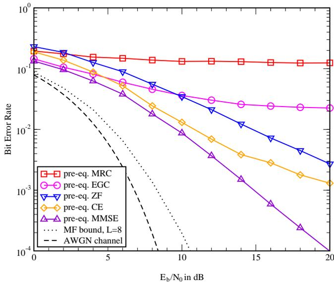
Fig. 2. Performance of basic OFDM-CDM power constrained pre-equalization techniques, spreading length  $L=8$ .
