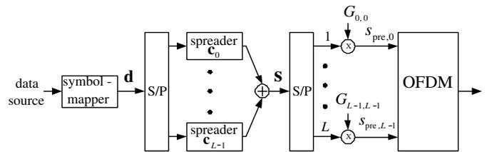
Fig. 1. OFDM-CDM transmitter with pre-equalization.
