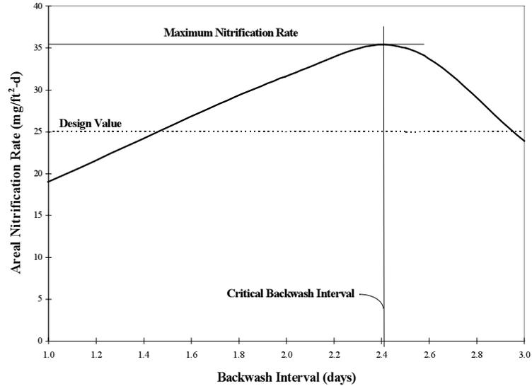
Figure 3. Critical backwash interval in a PBF (data from Chitta 1993).
