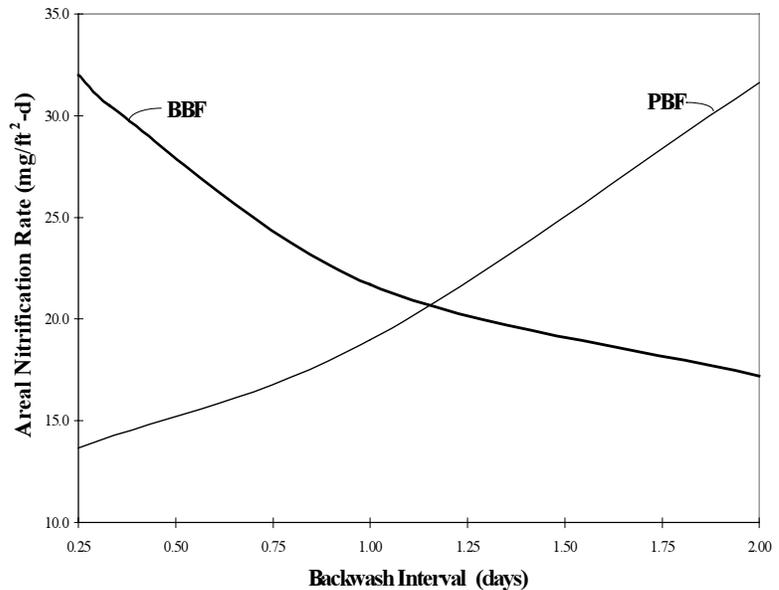
Figure 1. Nitrification rate as a function of backwash frequency (data from studies by Chitta 1993 & Sastry 1996).
