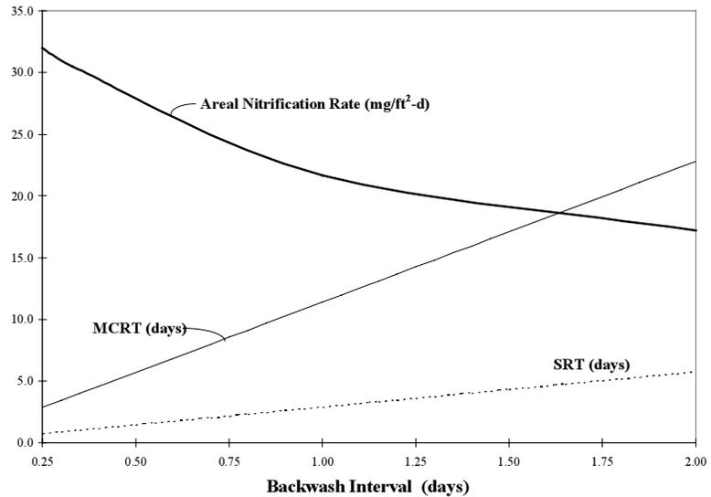
**Figure 4.** Areal nitrification rate and MCRT in a BBF ( $B_R = 0.8$ ). (nitrification data from Sastry 1996; 0.25 d interval from regression).
