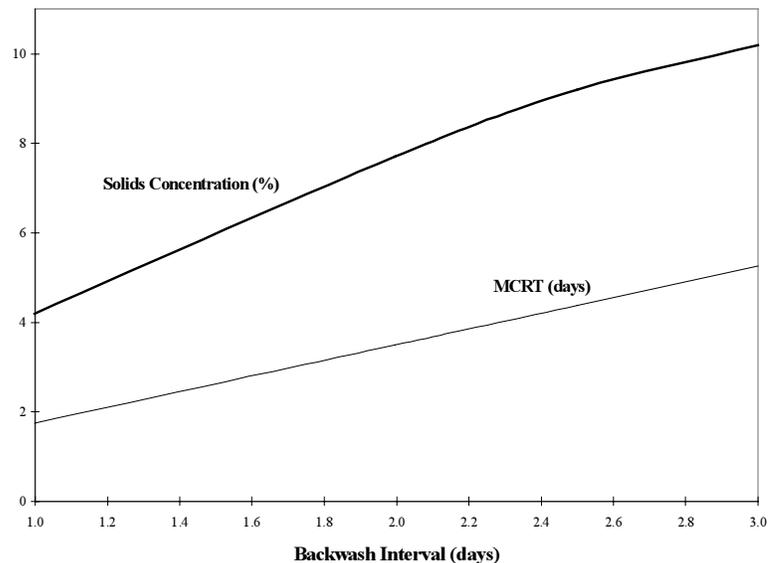
**Figure 2.** PBF mean-solids concentration and MCRT ( $B_R = 0$ ;  $SRT = MCRT$ ). Successful filter management is balancing the benefit derived from increasing MCRT with the escalating demands exerted by extending SRT, which increases the solids concentration.
