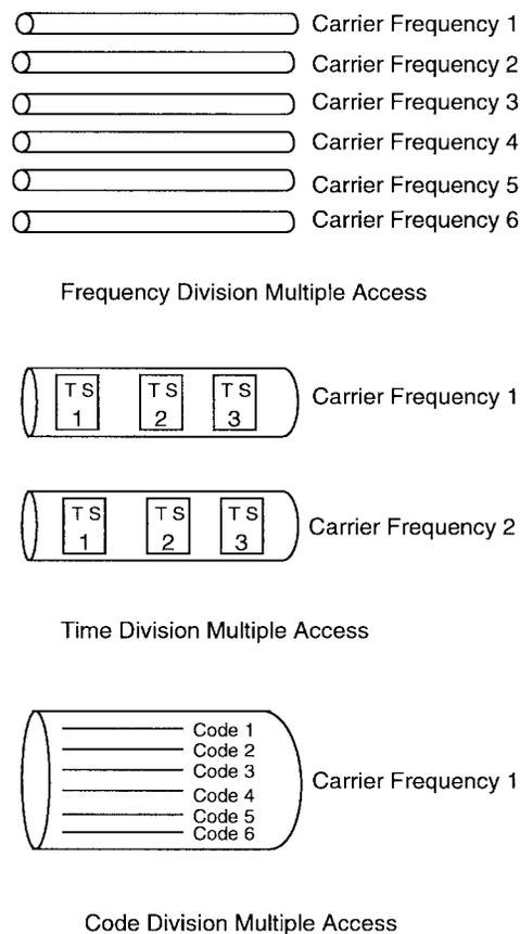
Fig. 2. Channel usage by FDMA, TDMA, and CDMA [12].
