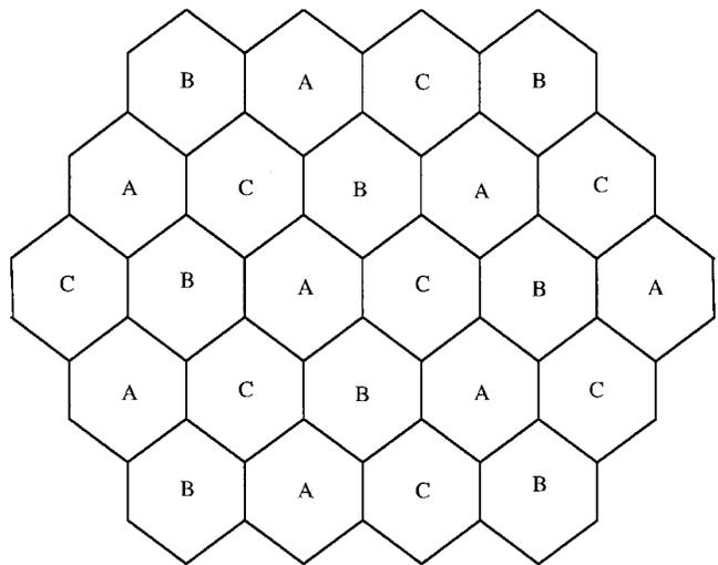
Fig. 3. Frequency assignment for cellular mobile communications.
