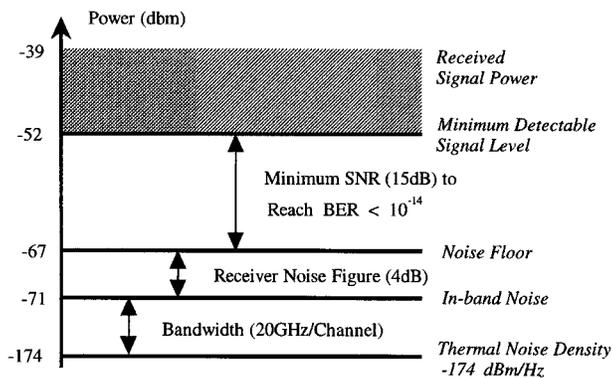
Fig. 13. Signal-to-noise budget for the intended RF/wireless interconnect system.
