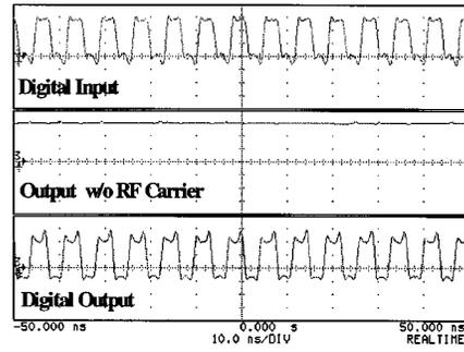
Fig. 22. Input and output waveforms of FDMA/CDMA-interconnect system with 5-GHz RF carrier.
