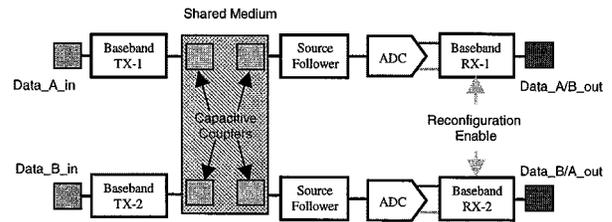
Fig. 18. Block diagram of  $2 \times 2$  baseband CDMA-interconnect system.
