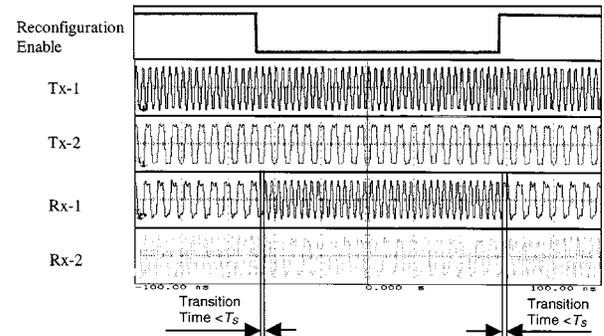
Fig. 19. Channels reconfigured seamlessly within one symbol period of  $T_s$  at  $F_c = 2.8\text{ GHz}$ .
