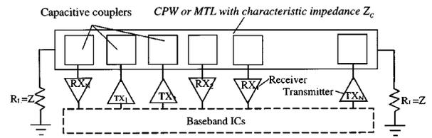
Fig. 5. A representative RF/wireless interconnect channel with multiple I/Os.
