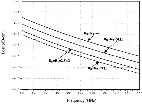
Fig. 7. Extra CPW attenuation caused by 20/20 shunted I/O transceivers.
