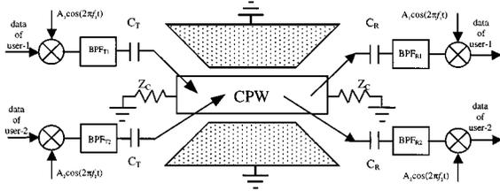
Fig. 8. Top-level schematic of a FDMA-interconnect.
