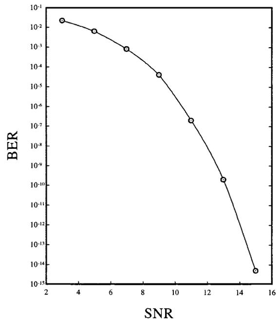
Fig. 12. BER versus SNR in CDMA-interconnect with 4 I/O subchannels.
