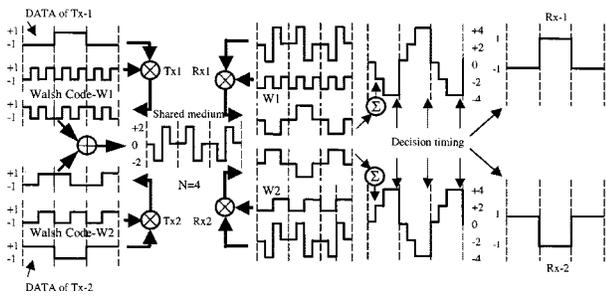
Fig. 10. Operation of a CDMA-interconnect with two I/O subchannels.
