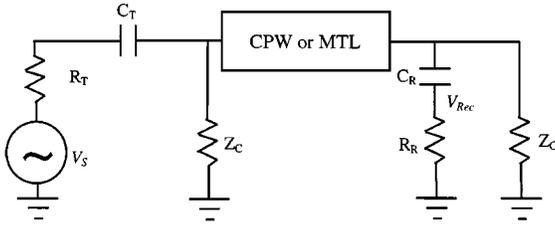
Fig. 6. Equivalent circuit for a representative transmitter-receiver loop.
