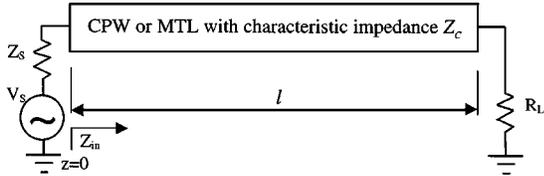
Fig. 4. CPW must be properly terminated with  $R_L = Z_C$  to minimize the frequency dispersion.
