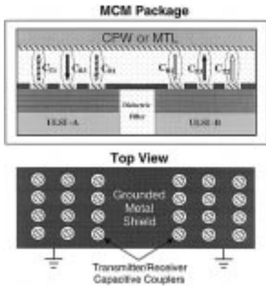
Fig. 3. ULSI chips communicate with each other through a miniature wireless LAN inside a MCM package.
