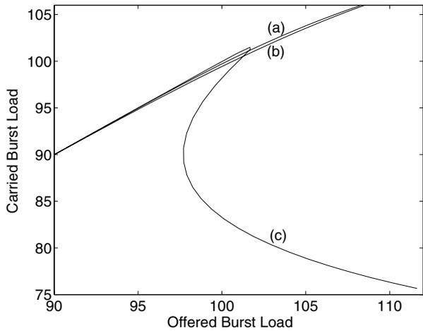
Fig. 5. Carried burst load  $(1 - P) \cdot \bar{\rho}$  against external load  $\bar{\rho}$  for an SD pair in a four-node symmetrical JET/OBS network with 120 wavelengths.
