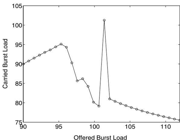
Fig. 1. Destabilising effect of deflection routing in a four-node symmetrical JET/OBS network.
