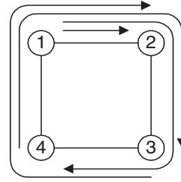
Fig. 3. Four-node symmetrical OBS network topology. Each arc represents a route traversing the link from node one to node two. Routes not traversing this link are not shown but can be deduced by symmetry.
