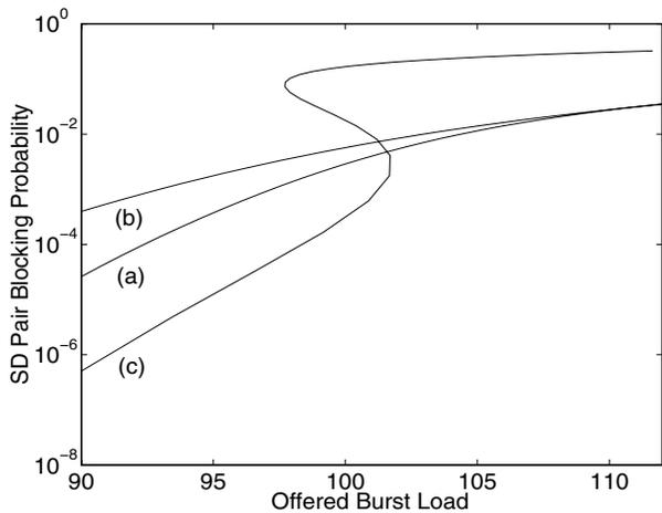
Fig. 6. End-to-end SD pair blocking probability  $P$  against external load  $\bar{\rho}$  in a four-node symmetrical JET/OBS network with 120 wavelengths.
