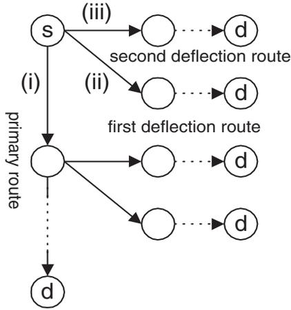
Fig. 2. Primary route with deflection routes for an isolated SD pair. To satisfy properties (a) and (b), links (i), (ii) and (iii) are chosen to be distinct. The first deflection route is chosen as the shortest route from the source to the destination that does not traverse link (i). The second shortest route is chosen similarly but does not traverse both links (i) and (ii).
