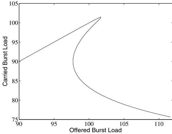
Fig. 4. Carried burst load  $(1 - P) \cdot \bar{\rho}$  against external load  $\bar{\rho}$  for an SD pair in a four-node symmetrical JET/OBS network with deflection routing.
