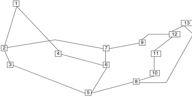
Fig. 7. Sample OBS network: NSFNET T3 comprising 13 OXCs and 32 directed links containing one fibre, each comprising of 120 wavelengths. We evaluate the performance of this sample OBS network for order-one and order-two deflection schemes with wavelength reservation.
