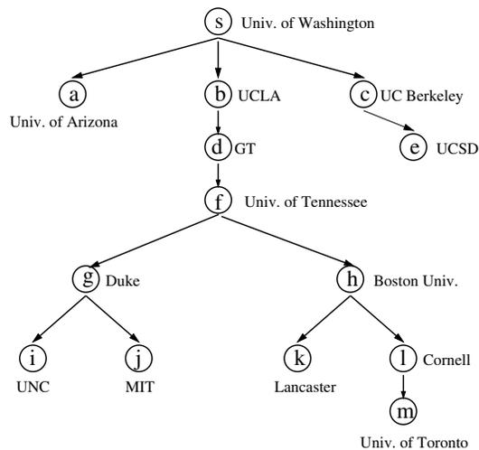
Fig. 12. Single Source Widest-Path Tree rooted at UW
