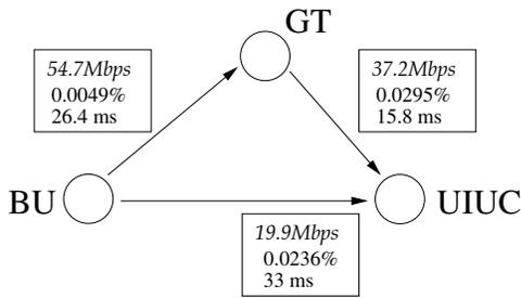
Fig. 11. Throughput Improvement on Chains of TCP
