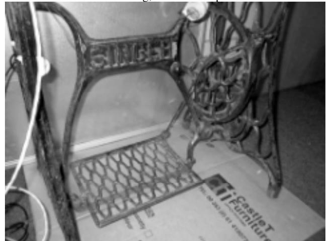
Figure 3. The sewing machine table, showing the pedal and wheel mechanism. A dynamo can be seen mounted near the top of the wheel.
