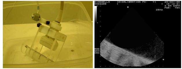
Figure 6. Left: the calibration phantom with the probe and Polhemus sensor attached. Right: a calibration image
