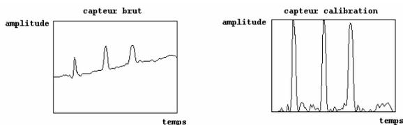
Figure 2. A sensor output before (left) and after (right) calibration
