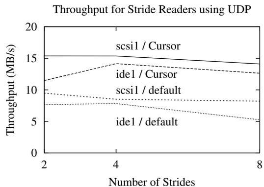
Figure 8: Throughput using the default NFS read-ahead compared to the cursor read-ahead, for reading a 256 MB file using 2, 4, and 8-stride patterns. *scsi1* runs 60-70% faster for all tests when cursors are enabled. *ide1* is only 50% faster for the 2-stride test with cursors enabled, but 140% faster for the 8-stride test.
