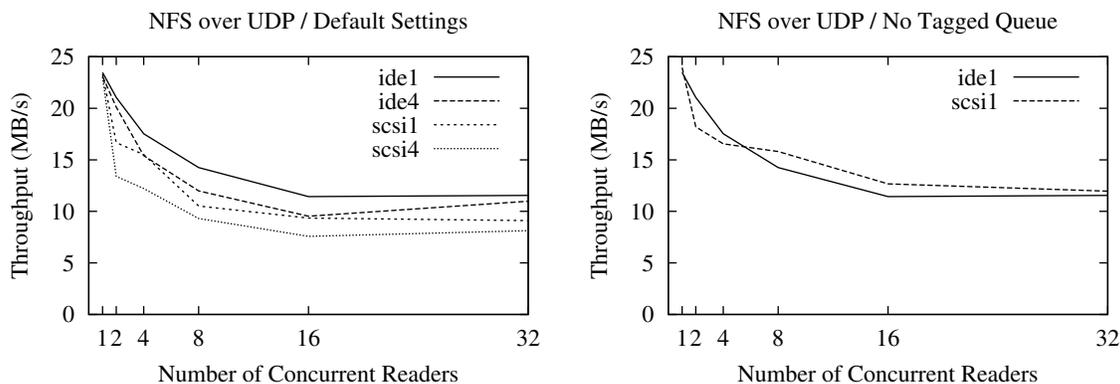
Figure 4: The speed of NFS over UDP, with and without tagged queues. Performance drops quickly as the number of concurrent readers increases. With tagged queues disabled, *scsi1* performance improves relative to *ide1* as the number of concurrent readers increases. Note that the ZCAV effect is still visible.
