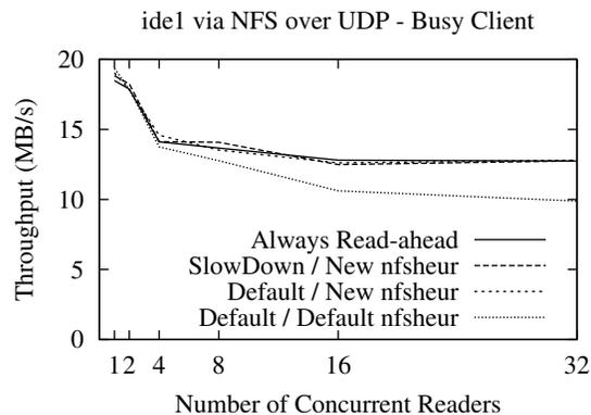
Figure 7: The effect of *SlowDown* and the new *nfsheur* table for sequential reads for disk `ide1` over UDP. The new *nfsheur* increases throughput for more than four concurrent readers, and gives performance identical to the Always Read-ahead case. *SlowDown* makes no further improvement.
