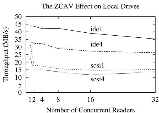
Figure 1: The ZCAV effect. The `scsi1` and `ide1` partitions use the outermost cylinders of the disk, while the `scsi4` and `ide4` use the innermost. As a result, the transfer rates for the `scsi1` and `ide1` partitions are higher than `scsi4` and `ide4`.
