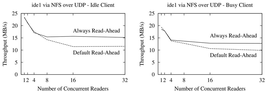
Figure 6: A comparison of the NFS throughput for the default read-ahead heuristic and a hard-wired “always do read-ahead” heuristic. All tests are run using file system `idle1` via UDP. The idle client is running only the benchmark, while the busy client is also running four infinite loop processes.
