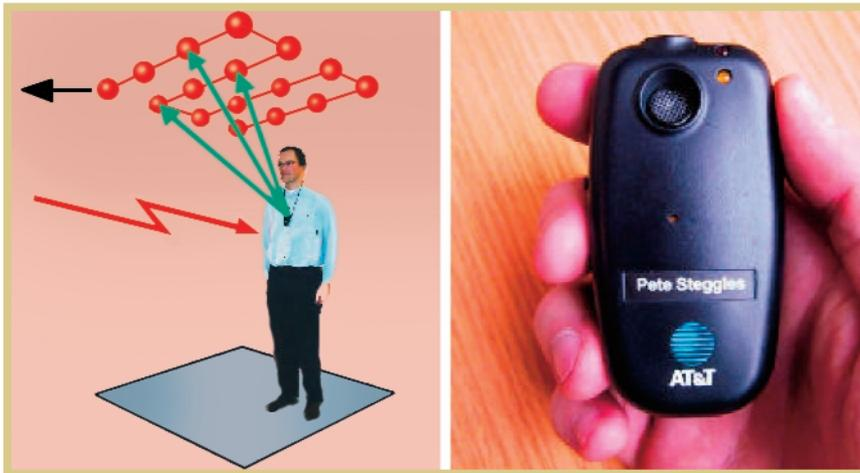
Figure 1. (a) The AT&T Active Bat system and (b) the Bat wireless tag device. Figure courtesy of M. Addlesee, R. Curwen, S. Hodges, J. Newman, P. Stegglas, A. Ward, and A. Hopper.<sup>7</sup>
