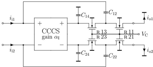
Fig. 3. Balanced-signal current-mode single-amplifier biquad containing a current amplifier with a negative gain  $\alpha_I$ .
