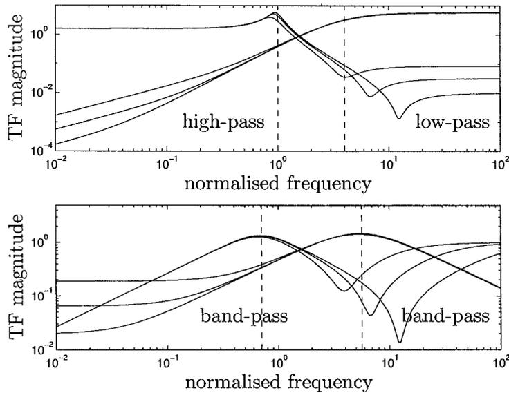
Fig. 2. Ideal transfer functions (TF) of the four basic Sallen-and-Key filters. The dashed lines indicate the different pole frequencies that were used to make all lines visible.
