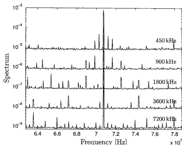
Fig. 12. Measurement of the intermodulation of signals with different frequencies with the power ripple caused by the charge pump (the spectrum units are chosen arbitrarily such that all peaks are visible).
