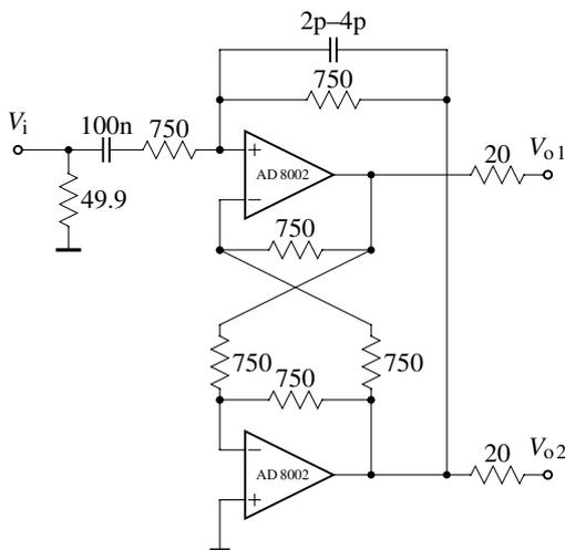
Fig. 10. Single-ended-to-balanced voltage converter using AD 8002 CFB opamps.
