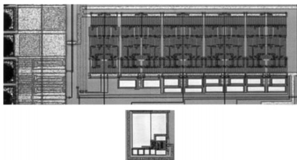
Fig. 9. Chip photos of the 7th-order filter and the charge pump (both photos have the same scale).
