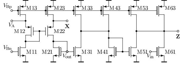
Fig. 6. Half circuit of the balanced current amplifier.
