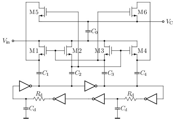
Fig. 8. Self-oscillating charge pump.
