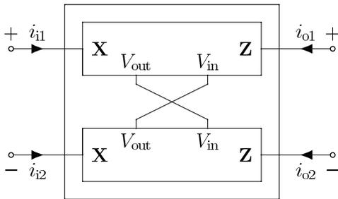
Fig. 5. Block diagram of a balanced current amplifier.
