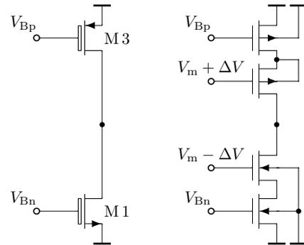
Fig. 4. Composite transistors (simple cascodes).
