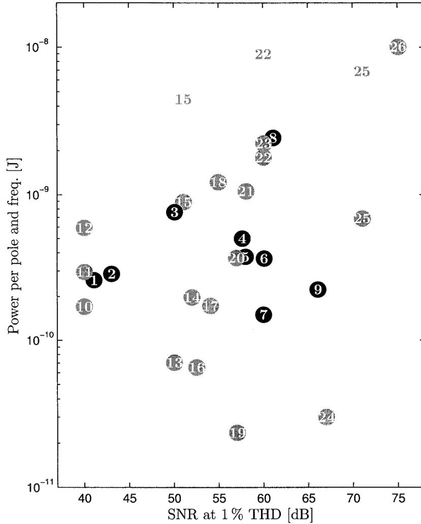
Fig. 13. Figure of Merit for different filters in the literature.
