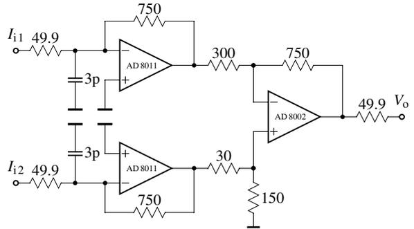
Fig. 11. Balanced-current-to-single-ended-voltage converter using AD 8002 and AD 8011 CFB opamps.
