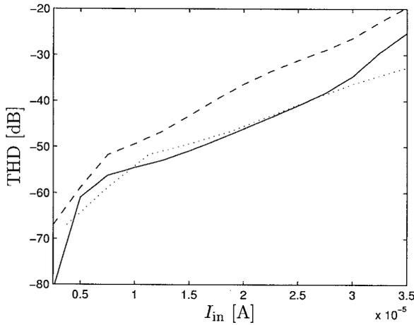
Fig. 14. Simulated THD of a conventional MOSFET-C SAB (solid), of a MOSFET-only SAB (dashed), and the latter curve with  $I_{in}$  scaled by 1.5 (dotted).
