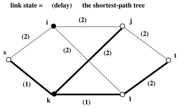
( d ) finding a delay-constrained tree from s to {j, l, t}
