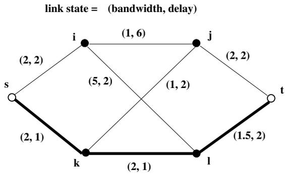
( a ) finding a bandwidth-delay-constrained path from s to t
