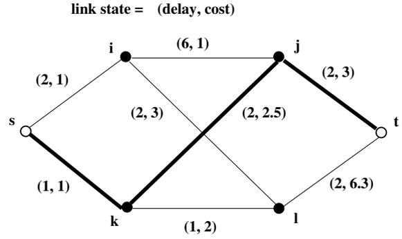
( b ) finding a delay-constrained least-cost path from s to t
