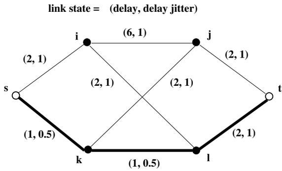
( b ) finding a delay-delayjitter-constrained path from s to t
