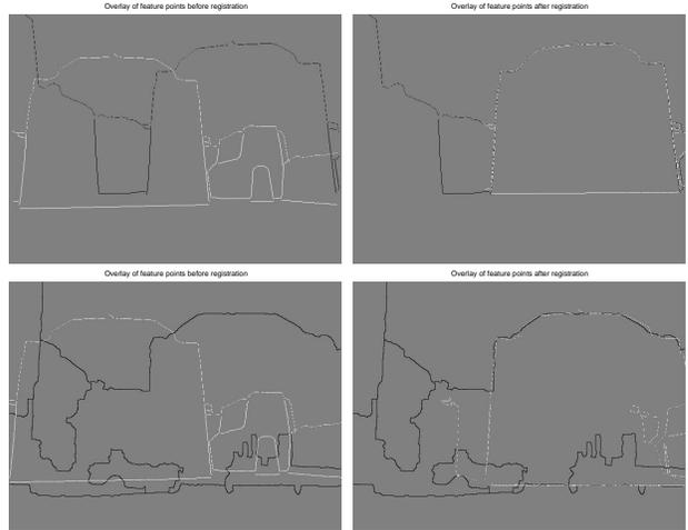
Figure 5: Overlay of feature points before and after registration. Top: Depth map with Depth map, Bottom: Depth map with Intensity image
