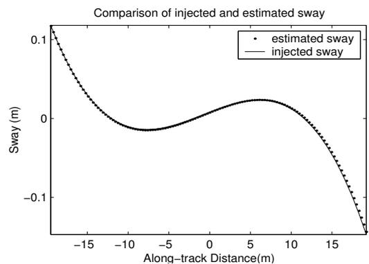
Figure 5: Comparison of estimated and injected fifth-order polynomial path distortions. The maximum estimation error  $\approx 3.5$  mm  $\equiv \lambda/14$ .
