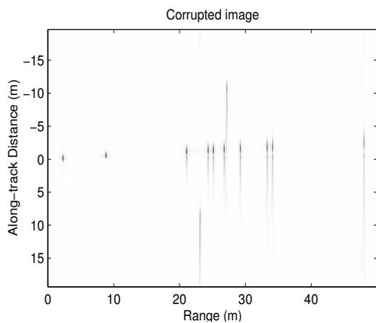
Figure 2: Reconstructed simulated scene showing the blurring to a number of point targets caused by a polynomial path distortion.
