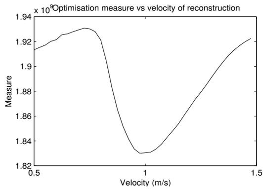
Figure 1: Optimisation measure as a function of varying the sonar speed employed in the reconstruction process. The data set is a bland clutter floor simulated at  $v = 1.0$  m/s.
