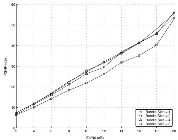
Fig. 12. PSNR performance for different sub-channel bundle sizes.
