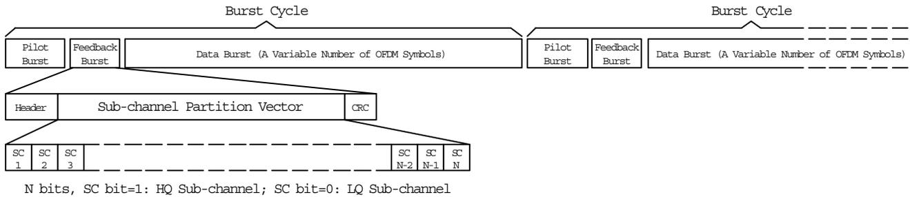
Fig. 4. Burst Structure.
