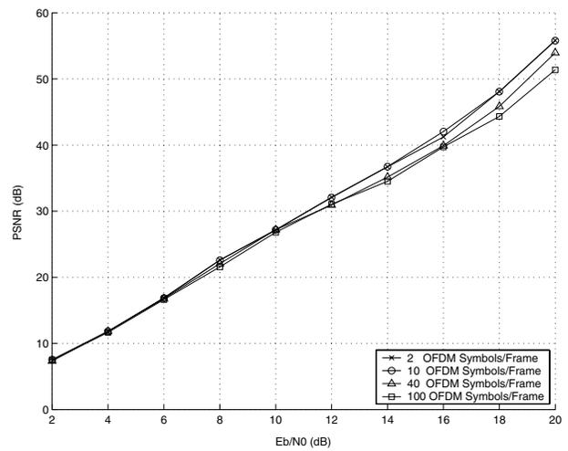
Fig. 11. PSNR performance for different frame sizes.
