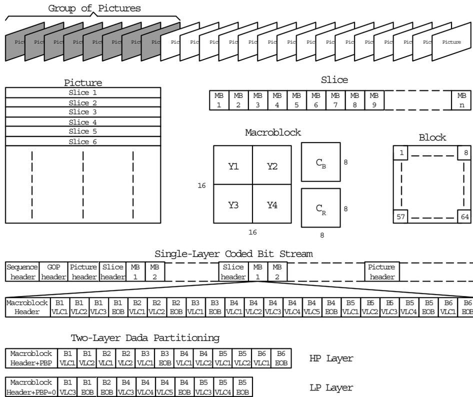
Fig. 1. Structure of MPEG data and data partitioning.
