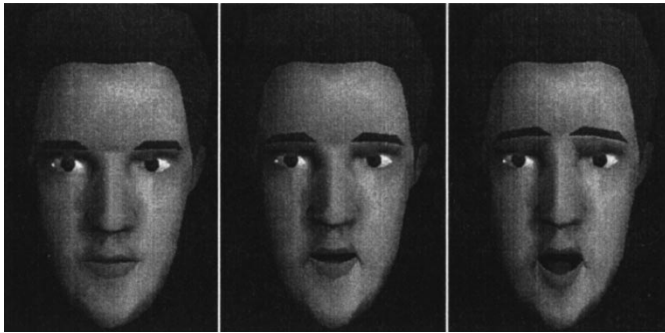
Fig. 13. FIT results for expression "surprise." Only expression FAP is sent for each frame, and the 27 low-level FAP's are interpolated from it using FIT.
