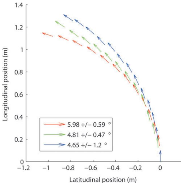
**FIG. 10.** Turning paths for 13 gait cycles of 3 successive runs. Locations and heading of the robot were recorded at the same point in the gait cycle from experimental videos. Color images available online at [www.liebertpub.com/soro](http://www.liebertpub.com/soro)
