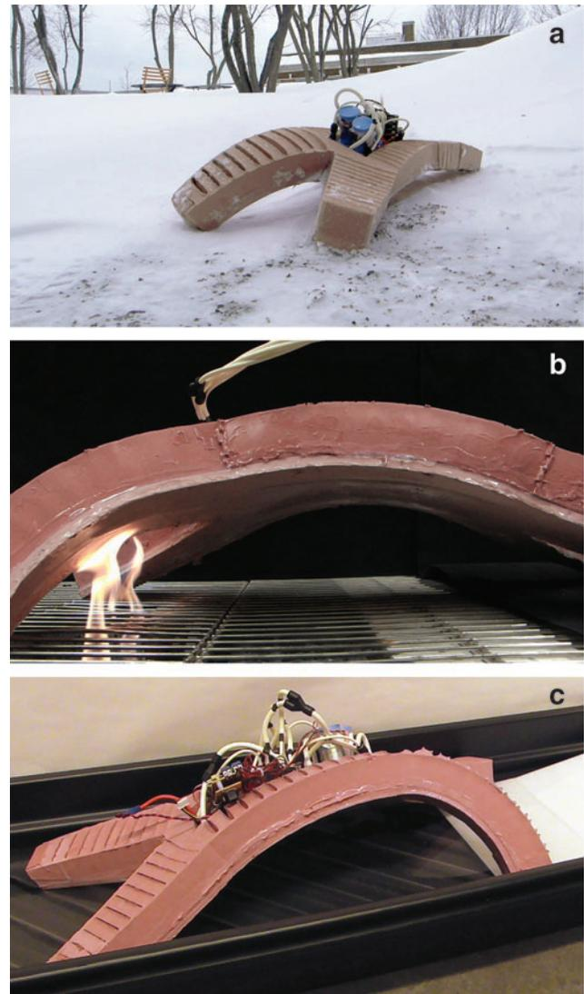
**FIG. 11.** Resilience of the untethered soft robot to harsh conditions. (a–c) Images from experiments of the soft robot operating untethered in a variety of harsh conditions, including a snow storm (a), a fire (b), and water (c). Color images available online at [www.liebertpub.com/soro](http://www.liebertpub.com/soro)
