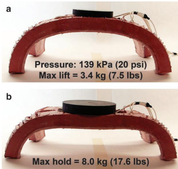
**FIG. 6.** Maximum lift and hold tests. **(a)** Starting from a flat position, a tethered version of the soft robot was able to lift a mass of 3.4 kg (7.5 lbs) when actuated with a pneumatic pressure of 139 kPa (20 psi). **(b)** Starting from an actuated position with an internal pneumatic pressure of 139 kPa (20 psi), the robot was able to hold 8.0 kg (17.6 lbs). Color images available online at [www.liebertpub.com/soro](http://www.liebertpub.com/soro)
