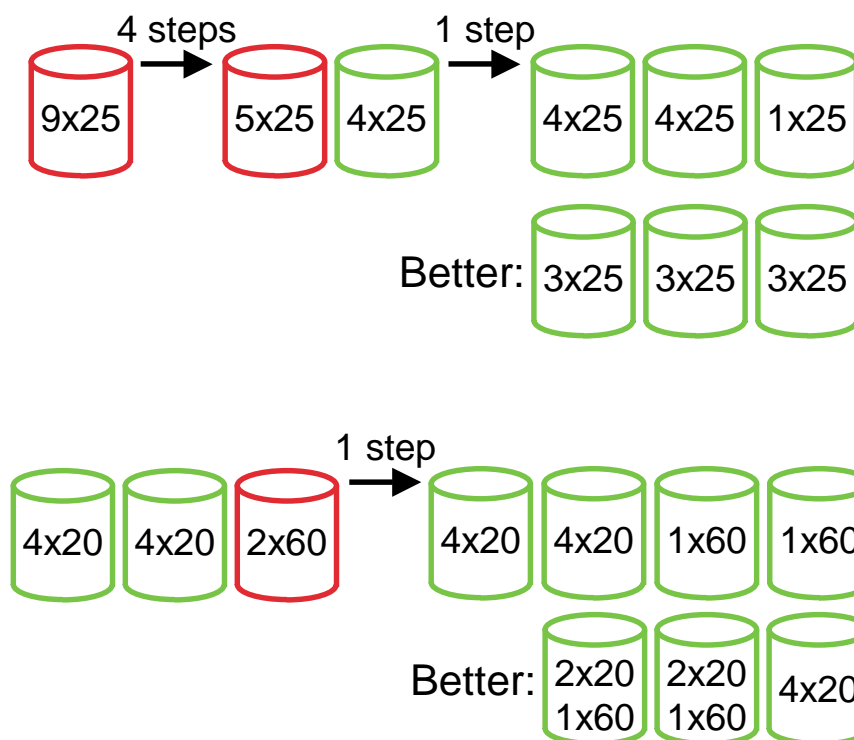
Figure 5.3: Problems with the simple loop. Each disk can handle 100 IOPS. The first example shows a failure of load balancing. The second example shows a failure to purchase a minimal number of disks. Stores are moved to available disks one at a time in this example.
