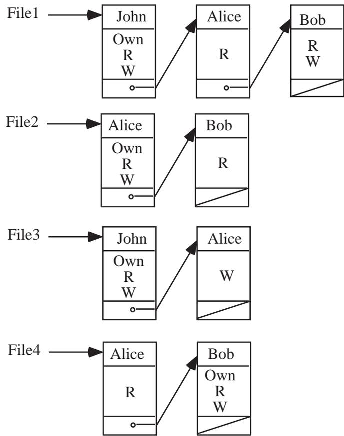
Figure 3: Access Control Lists for Files in Figure 1
