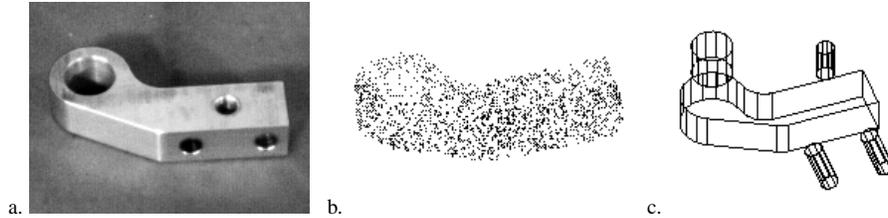
Fig. 1. Reverse engineering of a steering arm [Thompson et al. 1999]. a. Original part. b. Sensed 3D position points. c. Exploded view of the features making up the reverse engineered part.
